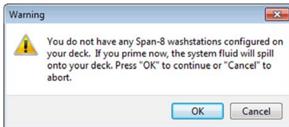
Figure 6.17 Warning to Address if a Span-8 Tip Wash ALP is Not Defined
