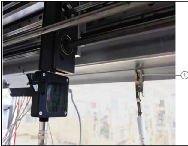
Figure 2.10 Span-8 Ground Connection to Side Arm Cover Screw
